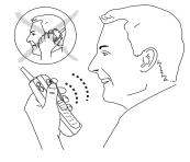
Press the Push-To-Talk (PTT) button to initiate a call in Radio Mode and press and hold the PTT button to speak. Use the top volume control to select radio audio volume.
